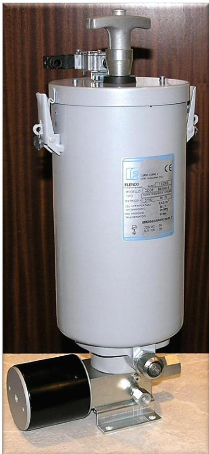
This pneumatic pump has a system operating pressure that is directly related to the air input pressure, the ratio being 45:1. The pump is energised by a 3/2 solenoid valve that must be ordered separately.
